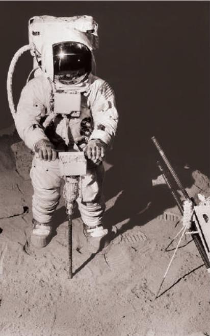
BLACK & DECKER developed a unique power head for drilling the lunar surface during the Apollo missions in 1971
