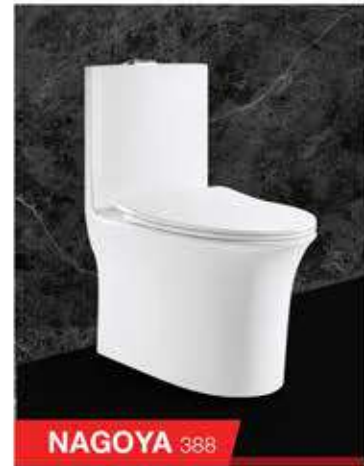
Siphonic one-piece toilet Bowl & Tank Size : 750 x 420 x 740 mm S-trap, 300 mm Roughing-in
