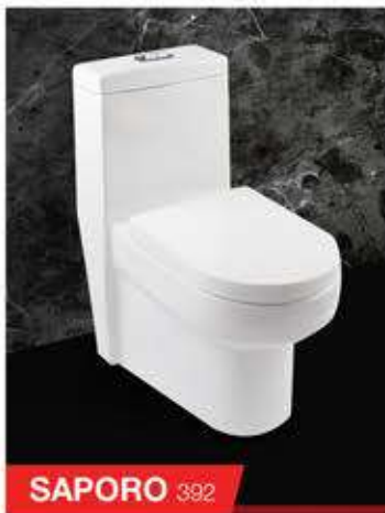
Siphonic one-piece toilet Size : 630 x 350 x 725 mm S-trap, 300 mm Roughing-in
