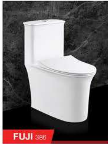
Siphonic one-piece toilet Bowl & Tank Size : 670 x 370 x 745 mm S-trap, 300 mm Roughing-in
