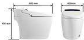
Automatic toilet Size : 680 x 400 x 495 mm S-trap, 300 mm Roughing-in
